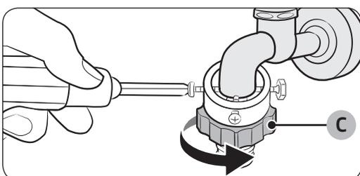
4. Insert the adaptor onto the water tap, and then tighten the screws while lifting the adaptor.
