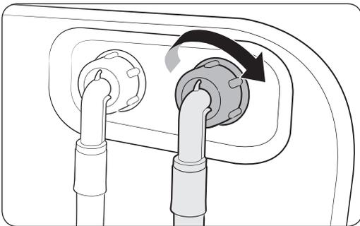
1. Connect the red end of the hot water hose to the hot water inlet on the back of the machine.
