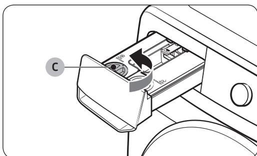
4. Turn the **auto softener compartment cover (C)** anticlockwise to open.
