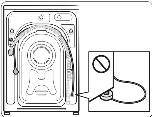
1. Gently slide the washing machine into position. Excessive force may damage the levelling feet.
