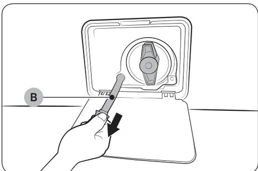
4. Open the tube cap and let water in the **emergency drain tube (B)** flow into the container.
