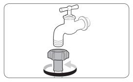
7. If you are using a screw type of water tap, use the provided screw-type adaptor to connect to the water tap as shown.
